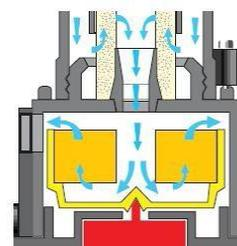
The polyurethane foam generates the flow and collects the dust.
